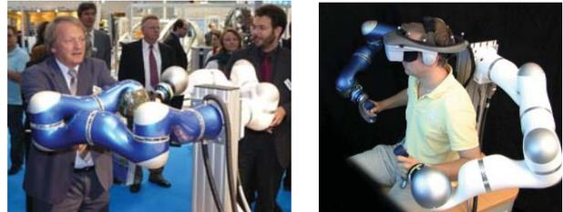
Fig. 1. Two-robot system providing bimanual haptic feedback. (left) Standard configuration, (right) Ergonomic configuration of the bimanual haptic interface.
